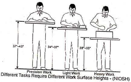
If the work surface is not adjustable, provide a platform for shorter workers or pedestals on the work surface to raise the work up for taller workers.
